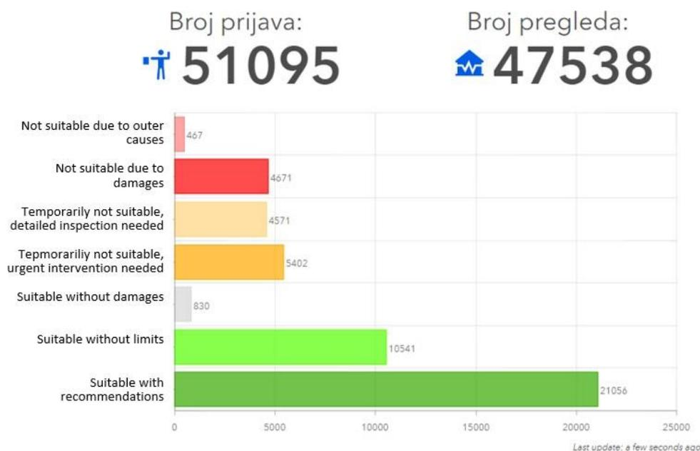
**Figure 1.15** Results of the damage estimates on buildings after the earthquake near Petrinja in the year 2020 on the 20 May 2021 (HCPI, 2021).
