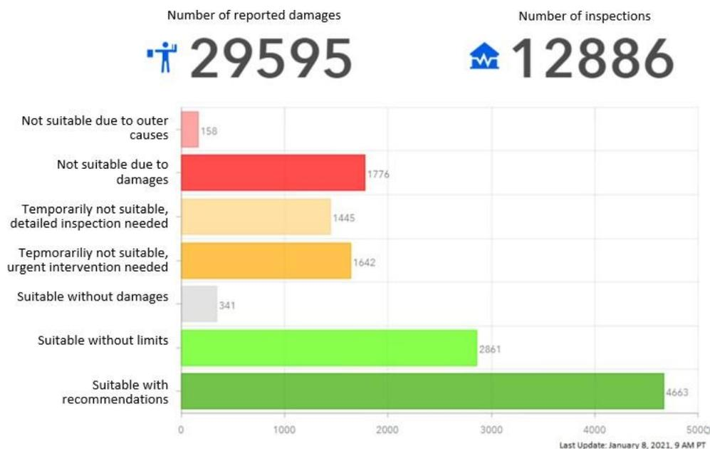
**Figure 1.14** Results of the damage estimates on buildings after the earthquake near Petrinja in the year 2020 on the 8 January 2021, 11 days after the main shock (HCPI, 2021).
